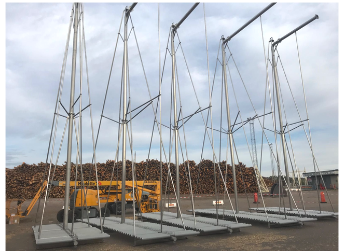
Systems extractable by crane with disc diffusers (on the left) and tubes (on the right)
