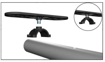
15. Next connect diffuser with upper saddle of clamp on saddle as shown.
