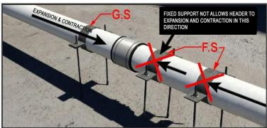
7. Maximum length of headers is 5.8m/20ft in length and header sections are connected with expansion joints. After the first expansion joint the first 2 supports are fixed support stand, the remainder are
