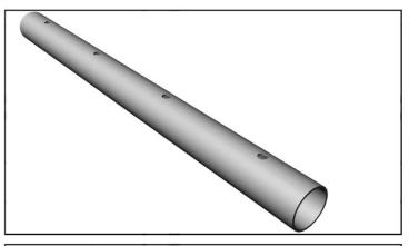
13. Make sure headers are drilled with 16mm holes.
