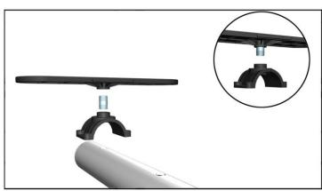
14. Install double nipple to the diffuser as shown.
