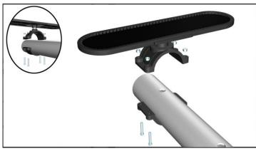
16. Then place diffuser assembly on pipe and at that time place lower saddle to the pipe as shown. Make sure diffuser assembly properly placed on drilled hole.
