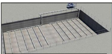
11. Complete installation of continuous purge (As an option).
