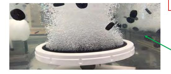
Loss of internal diffusion Lower efficiency Reduced organic removal rate
