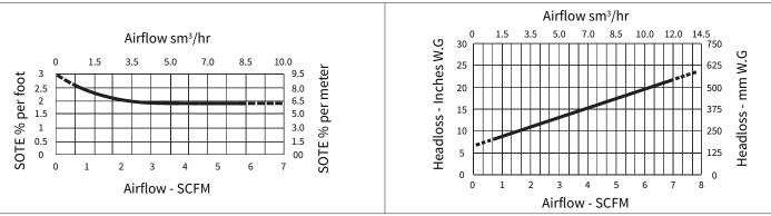
\*Installations under 2 SCFM/3.5m3/hr should consider an orifice plug to ensure uniform air distribution
