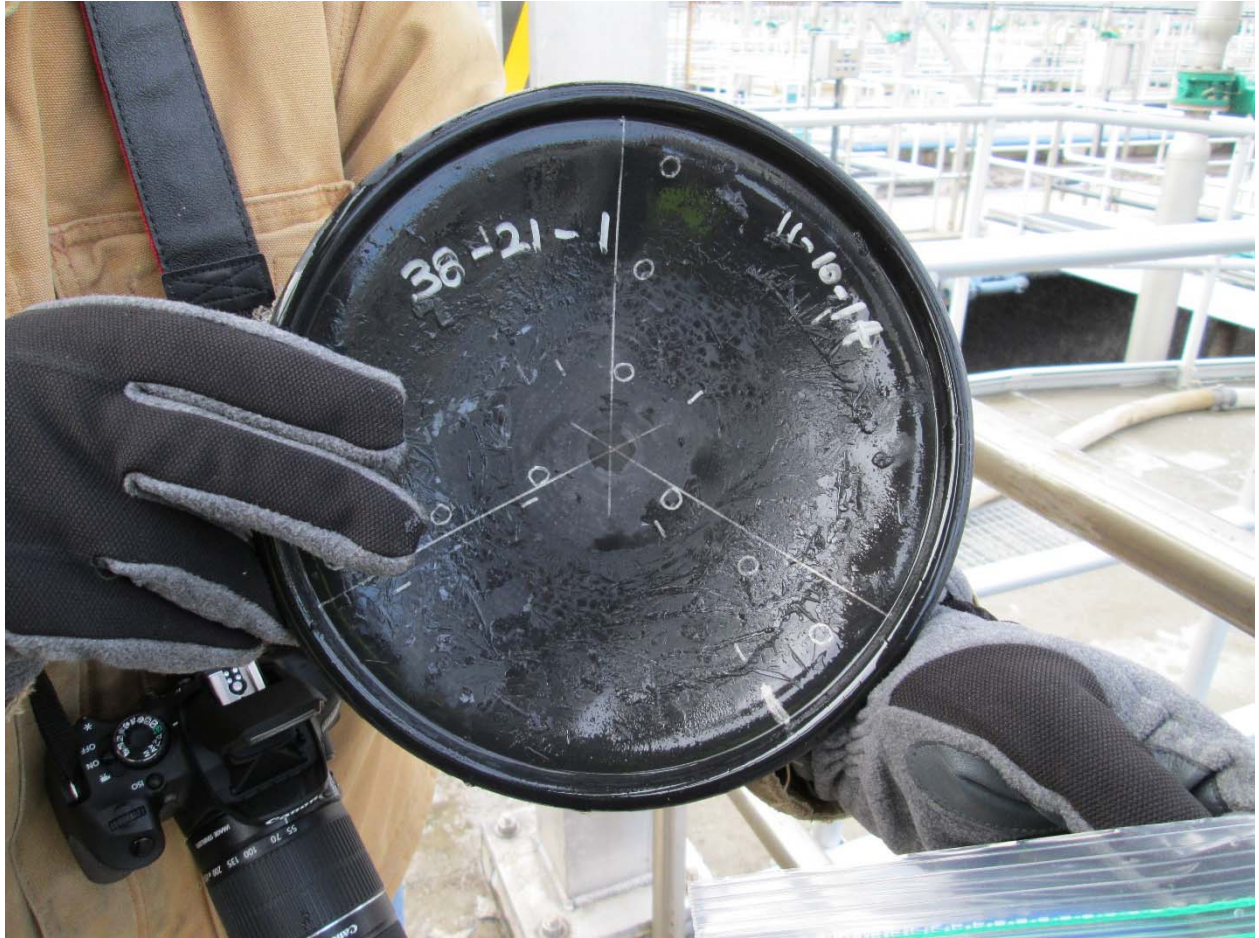
Figure 7: Close up of removed backside of pre-marked membrane for inspection and after spray washing.
