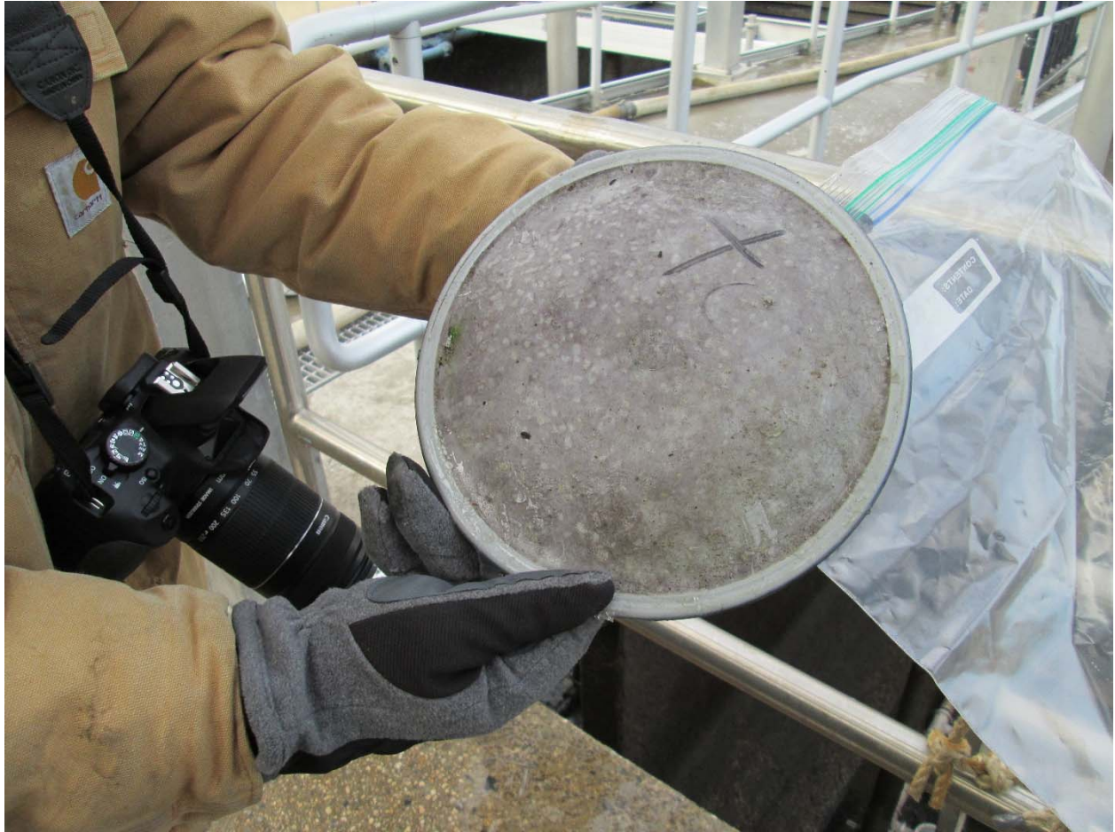
Figure 6: Close up of removed pre-marked tested PTFE face of membrane for inspection and after spray washing.
